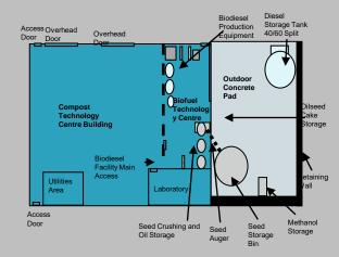
To ensure quality storage of biodiesel, a 10,500L split-tank storage system (60% petro-diesel and 40% biodiesel) designed to meet environmental safety considerations and to maintain the stored fuels at a temperature amenable to utilization and blending year round, regardless of outside temperature has been purchased. A blending ing system designed by Keller Equipment Supply Ltr
